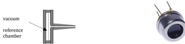
Fig 3, Principle of the absolute pressure sensor.
